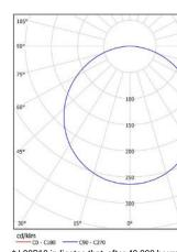
\* L80B10 indicates that, after 40.000 hours of functioning, 90% of the luminaires will have a lumen output of at least 80% of the initial value.
